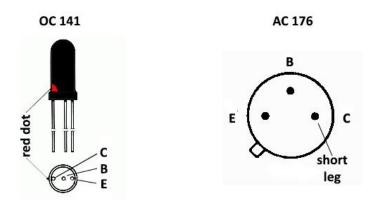
Be careful soldering transistors to the board. They don't like heat too much. I'd suggest keeping the leads long and sticking out 2 or 3 cm above the board (that's about an inch). This will act as a heat sink. Solder one lead and then wait a few seconds (solder the lead on the other transistor for instance).
