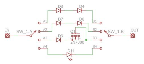
Note: I apologize for the weird numbering of the parts here. Diodes D4 and D8 may be replaced by jumpers is you want lower clipping threshold, for instance using a single germanium diode. Q1 is intended to be a 2N7000 mosfet. When using others like the BS170, beware of different pinouts. D9 should always be included.
